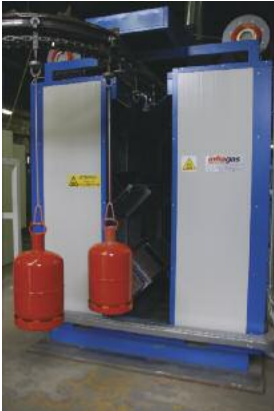
Powder paint infrared curing oven, for gas cylinders
