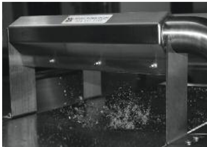
Centrifugal blowers and air knives made to dry, to clean and to cool metal sheets and parts in process
