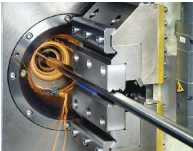
Guide bars made of Cerazur® Extremely high abrasion resistance, extremely high form stability
