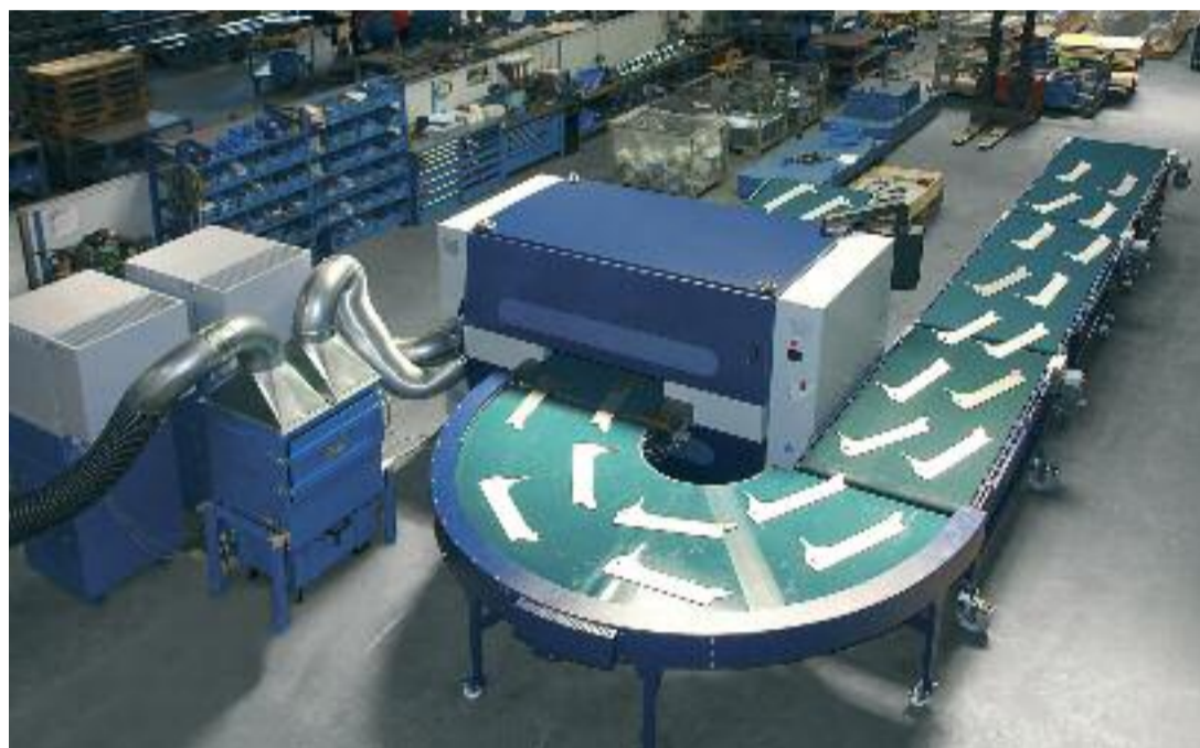
Lissmac deburring machine SBM-XL 1000 G2S2 with dust suction and transport belts
