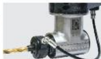
Re-Cool Nuts - Int. coolant option on angle heads supplied only for Ext. Coolant
