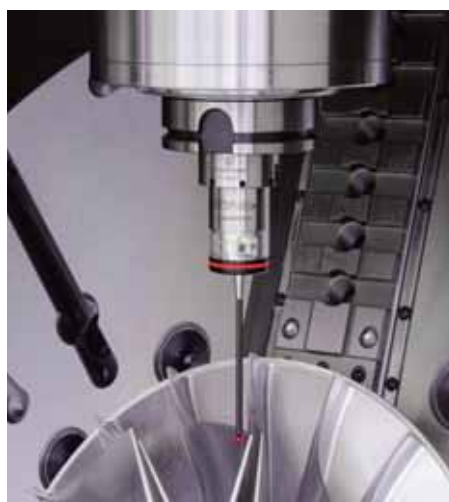
VOP40P: The high precision probe, with piezo-electric technology on board, for precise measurements on inclined surfaces
