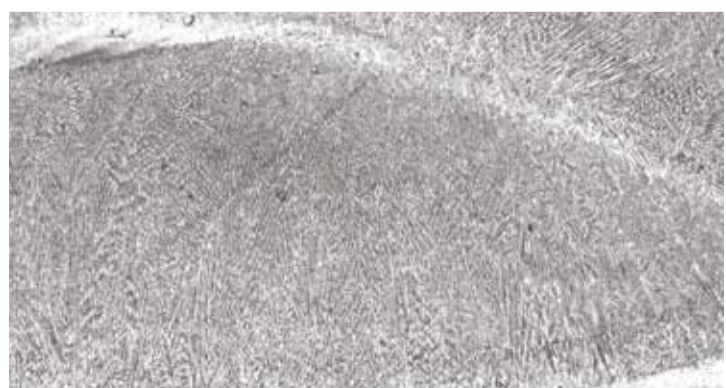
Fig. 41 - Microstructure of the fusion zone - B2
