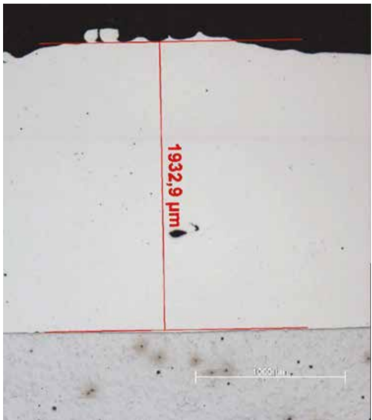
Fig. 35 - Detail of the repair thickness - A2
