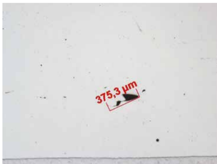
Fig. 39 - Detail of a fusion defect between the first and second repair passes - B2
